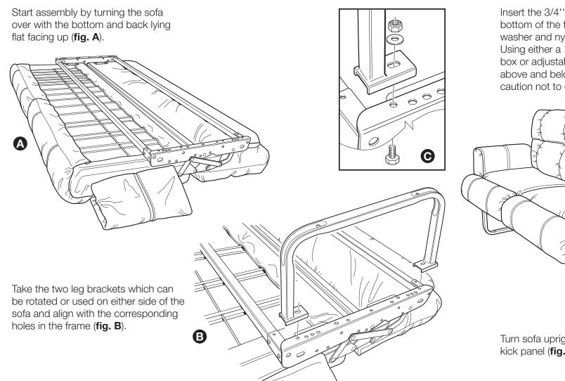
Insert the 3/4" length bolt through the bottom of the frame and attach the washer and nylock nut from the top. Using either a 1/2" socket, open-end, box or adjustable wrench from both above and below, tighten snuggly using caution not to overtighten (fig. C).
